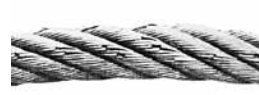
Two parallel rows of wire breakages caused by too small grooves in the rope sheaves.
